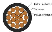
Extra fine bare copper conductor Polychloroprene rubber jacket
